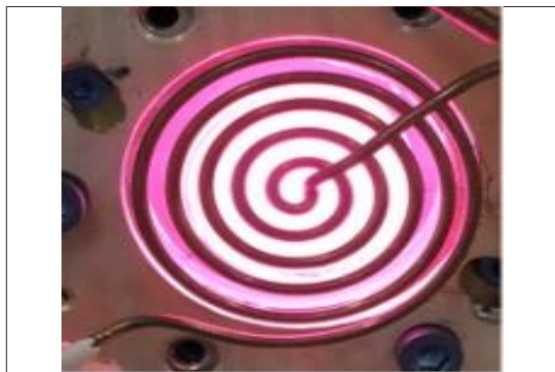
Fig.1 Ionization of hydrogen gas
