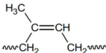
Fig. 2. Cis-1,4 polyisoprene (major component of natural rubber).
