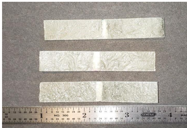
Figure 3: Tested E-Glass/Epoxy Composites Samples: Baseline (Bottom), 4 days (Middle), and 15 days (Top).
